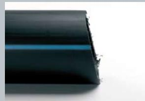
Pipe surface in the welding zone needs to be tightened when treated and the pipe ends had to be beveled. In order to obtain reliable welded joints it is of great importance to have clean surfaces. Clean surfaces to be welded with alcohol using fluffless absorbent paper.
