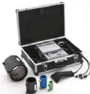
Polyvalent electrofusion welding unit with scanner barcode reader. 230V input power supply. Welding range 20÷160 mm. According to ISO 12176/2-3 Norms. Supplied in transport case.
