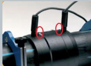
Welding indicator on the socket indicates if the socket has been welded.
